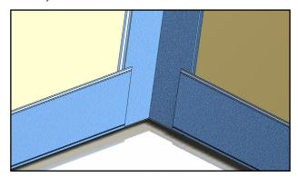
3. Finish the valley by applying 6" wide aluminum Foil Seal Tape on both sides of the valley bleeder so that the Sol-R-Skin™ BLUE aluminum completely seals and covers the valley section of the roof.
